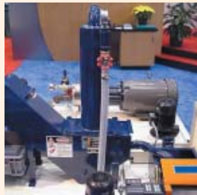
AT-Cleaner with Super Separator for sludge clean-out
