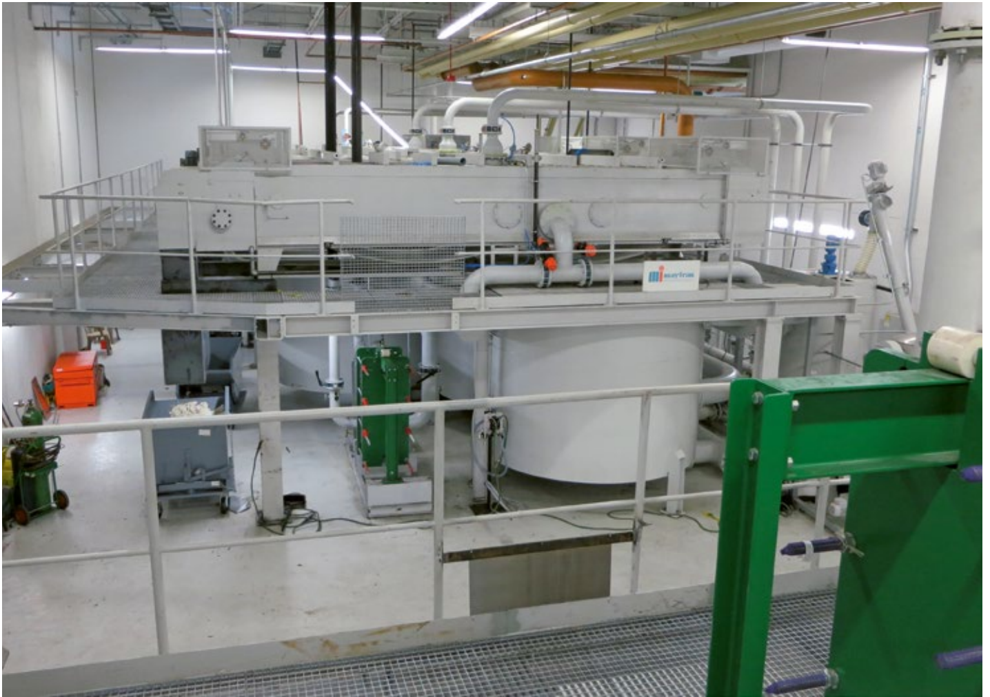
Pressure belt filter system consisting of several filter modules
