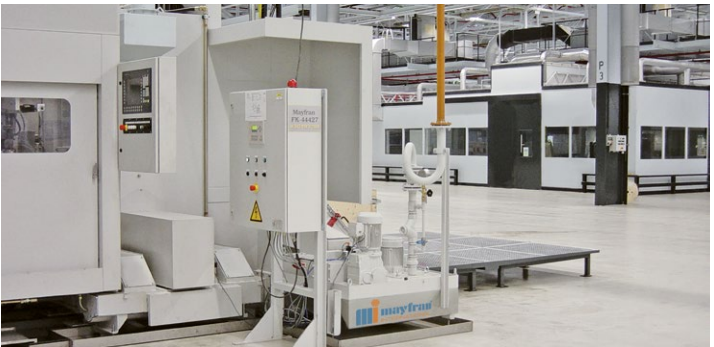
Machine pump station directly on the machine with supply to the Viavent overhead system
