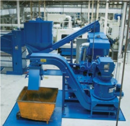
Centrifuge, chip crusher, conveyor and container loading
