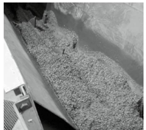
The push-bar centres automatically on the floor of the conveyor trough.
