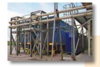
Bulk filling trailers are one of the options available for chip collection. Comprising of reverse onto fill pipework the system has auto fill sensors, trailer changeover divertors, docking steelwork.
