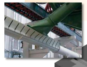
Bespoke telescopic sections to allow for vertical Z axis travel complete with linear actuator, precision bearing slideways, gauge length measurement & close tolerance ptfe/nylon air seals.
