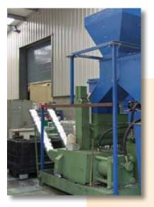
Briquetter unit with hydraulic power pack, inlet feed screw & PLC control.
