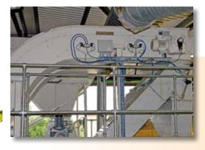
Product feed chutes that are suitable for multiple conveyors. Available with pneumatic divertors, sound dampening liners and bin fill level sensing devices.
