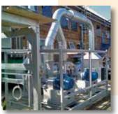
Air separation cyclone unit having a heavy duty mild steel construction complete with removable wear liners to suit applications.
